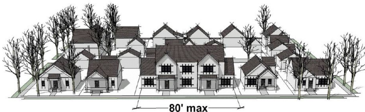
Figure 2-19: Maximum Allowable Length of Multi-Family Residential Structure
